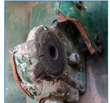
Severely damaged gladhand & seal
