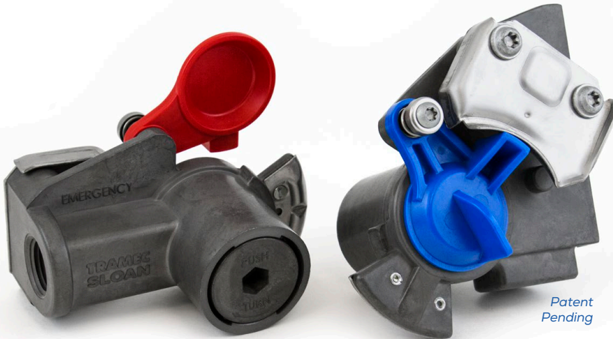
Maintenance is easy and requires only a 3/8" hex key.
